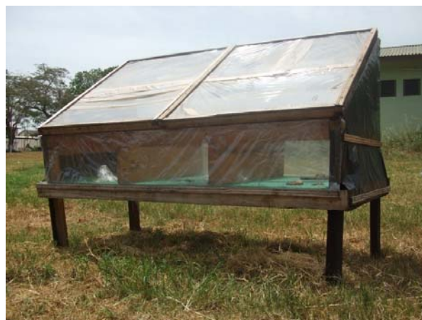
Figure-4. Panel D with the black polythene sheet covering the two opposite sides
