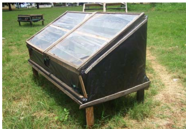
Figure-2. Panel B with three of its sides covered with black polythene sheet.
