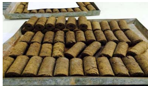
Figure-1. The green charcoal sticks in dry condition.
