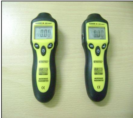
**Figure 5.** Microwave radiometer.
