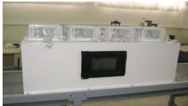
**Figure 4.** Mounting conveyor belt and microwave tunnel.
