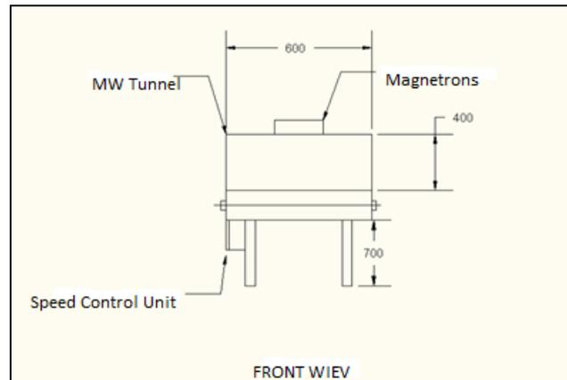
**Figure 3.** Front-view of conveyor belt and microwave tunnel.
