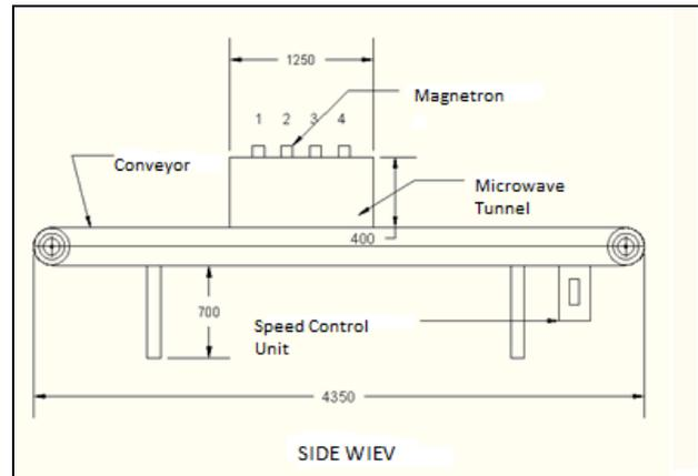
**Figure 2.** Side-view of conveyor belt and microwave tunnel.
