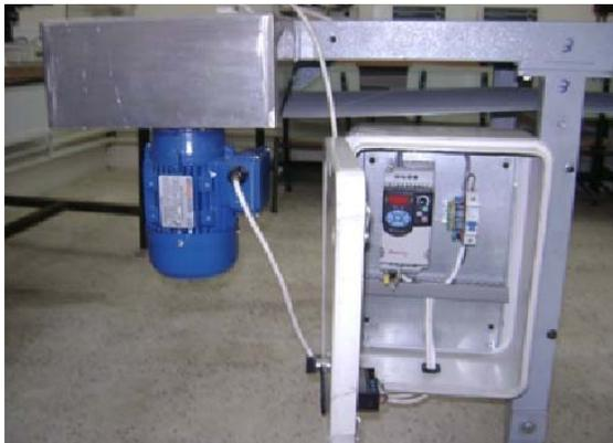
**Figure 1.** Conveyor belt, electric motor and speed driver.
