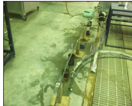
**Figure-2.** Laboratory evaluation of the laterals used for the tested irrigation systems.
