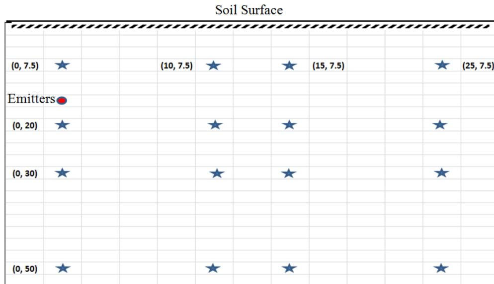
**Figure-5.** Sampling locations with respect to the Emitters for soil moisture measurements for both the SIS-15 and the KISSS-15.
