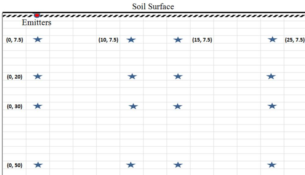
Figure-4. Sampling locations with respect to the Emitters for soil moisture measurements for the SDI system.
