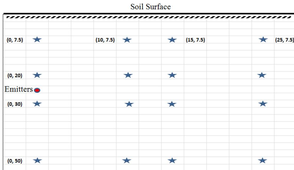
**Figure-6.** Sampling locations with respect to the Emitters for soil moisture measurements for both the SIS-25 and the KISSS-25.
