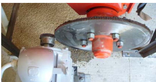
Figure-7. The contacts between designed gears and the seed drill.
