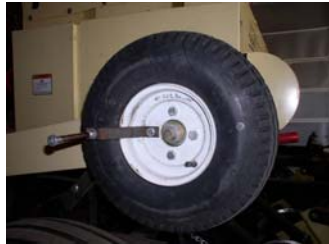
Figure-2. Calibration of seed drill could be done by driving feeding shaft manually [15].
