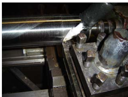
Figure-1b. Photographic view of the experimental set-up. Nozzle injecting liquid nitrogen.
