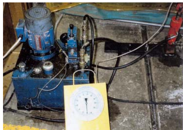
Plate-2: Hydraulic Power Pack
