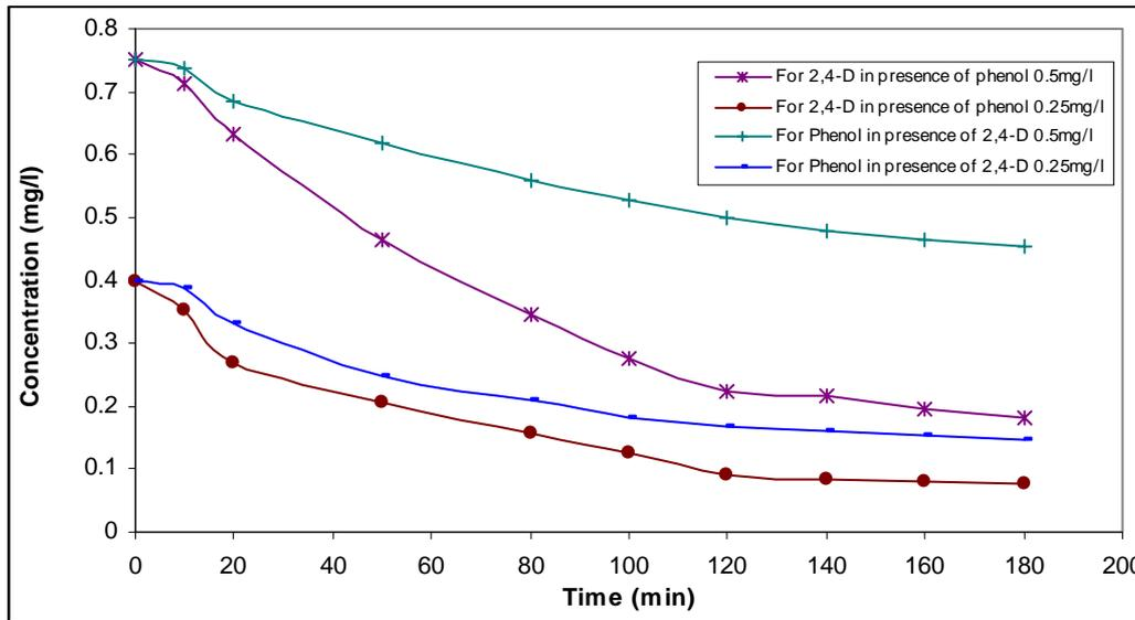
Figure- 2. Competitive sorption of 2,4-D and Phenol in presence of Phenol and 2,4-D, respectively.
