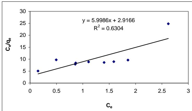
**Figure-4.** Application of Langmuir model for phenol sorption on waste tyre rubber granules.
