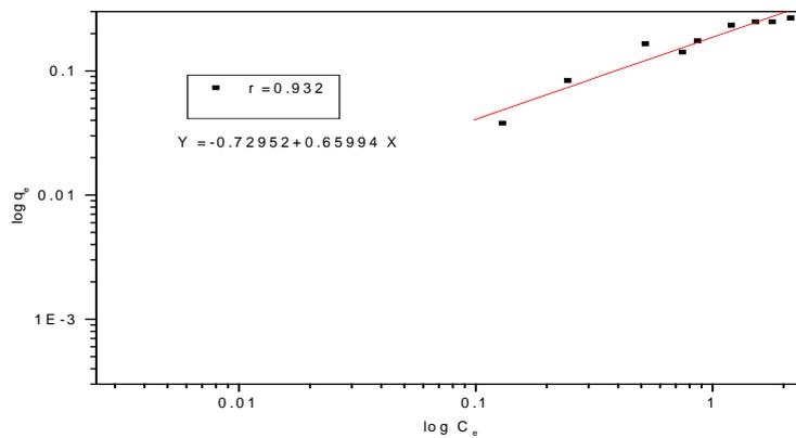
**Figure-5.** Application of Freundlich model for 2,4-D sorption on waste tyre rubber granules.
