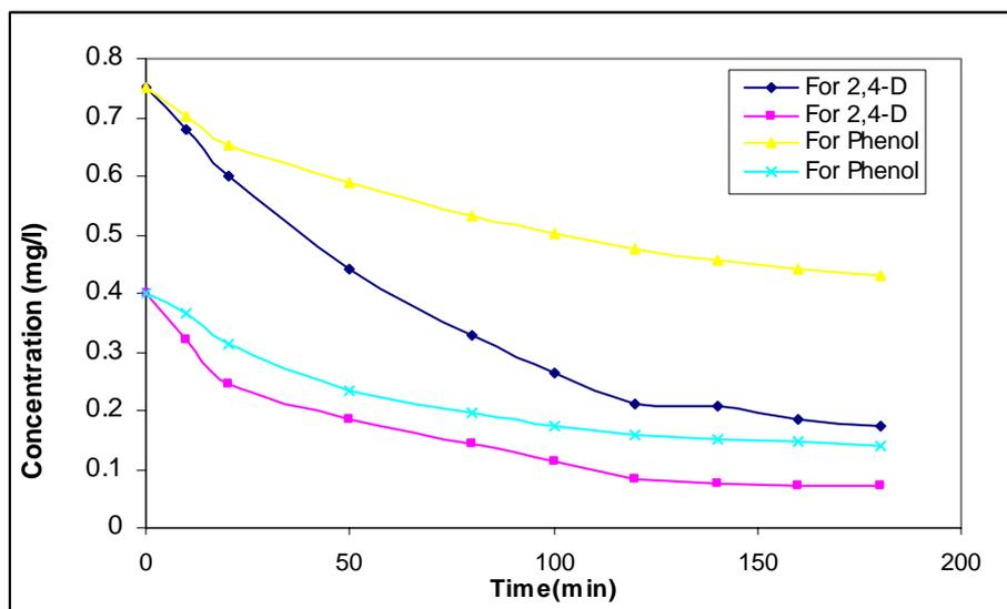
**Figure-1.** Change of concentration with time for 2,4-D and phenol sorption on rubber granules with initial concentration of 0.75mg/l and 0.4mg/l.
