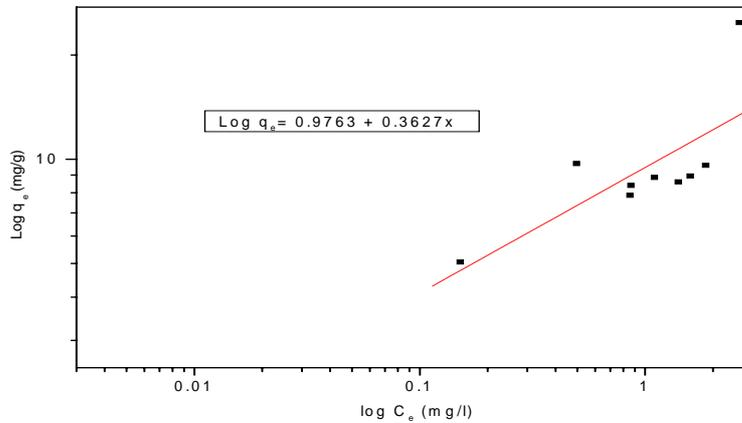
**Figure-6.** Application of Freundlich model for phenol sorption on waste tyre rubber granules.
