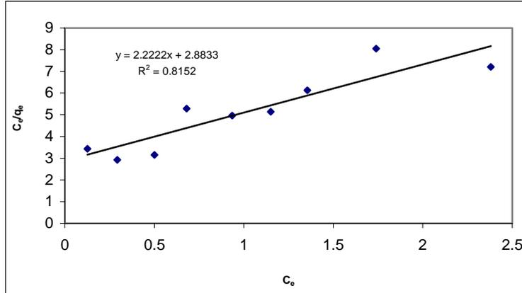
**Figure-3.** Application of Langmuir model for 2,4-D sorption on waste tyre rubber granules.
