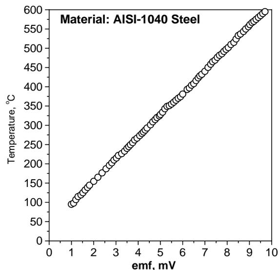
**Figure-4.** Tool-work thermocouple calibration curves.
