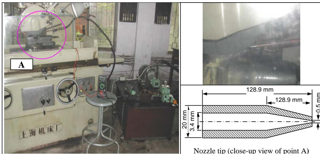
**Figure-1.** Photographic view of HPC jet delivery nozzle injecting cutting oil during grinding
