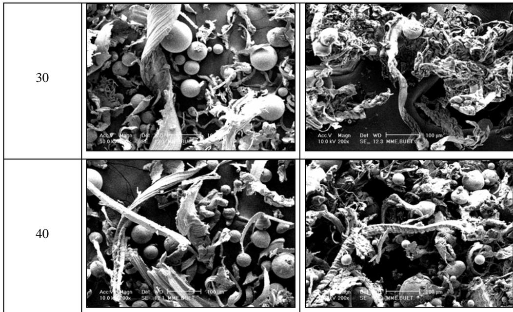
**Figure-3.** SEM photographs of grinding chips at different infeeds under (a) dry and (b) HPC conditions.
