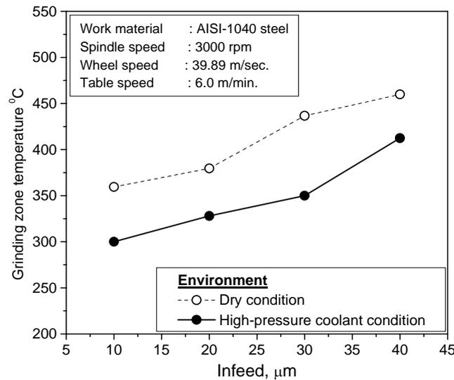
**Figure-5.** Variation in the grinding zone temperature with infeed under dry and high pressure coolant conditions.
