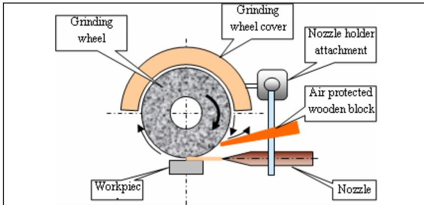
**Figure-2.** Schematic view of the nozzle positioning of the grinding wheel.
