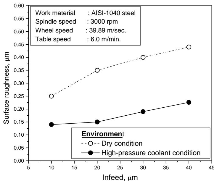
**Figure-6.** Variation in the surface roughness with infeed under dry and high pressure coolant conditions.
