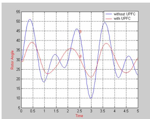
**Figure-15.** Swing curves-Classical model: Fault at bus # 26, no line cleared, UPFC in line # 26-29.
