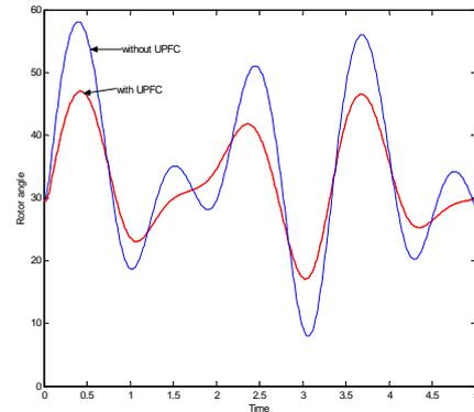
**Figure-11.** Swing curves –Fault at bus#26, no line cleared, UPFC in line 14-15.
