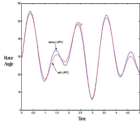
**Figure-12.** Swing curves –Fault at bus #26, line cleared 26-28, UPFC in line 26-29.
