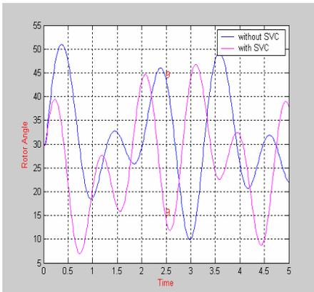
**Figure-13.** Swing curves- Classical model: Fault at bus # 26, no line cleared, SVC at bus # 28.
