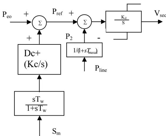
Figure-5. Controller structure for  $V_{seq}$
