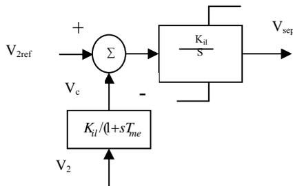
Figure-4. Controller structure for  $V_{sep}$
