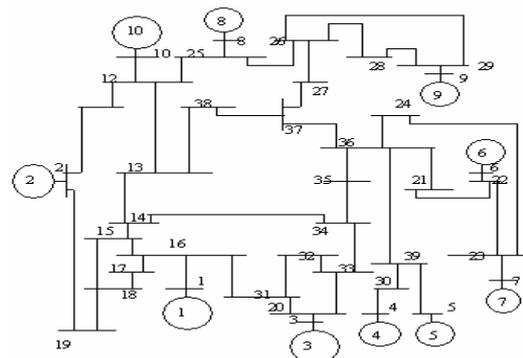
Figure-7. 10-Generator, 39-Bus, New England Test System.
