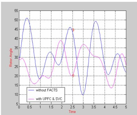
**Figure-14.** Swing curves- Classical model: Fault at Bus # 26, no line cleared, UPFC in line # 26-29 and SVC at bus # 28.
