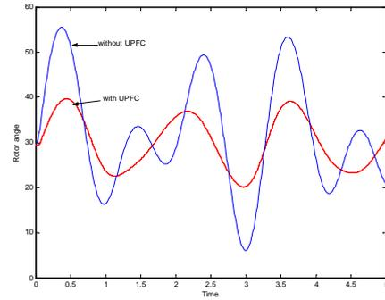
**Figure-10.** Swing curves: Fault at bus#26, no line cleared, UPFC in line 26-29.
