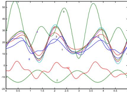
**Figure-8.** 11 Swing curves of generators #1 to # 10.
