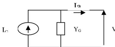
Figure-1. Stator representation.
