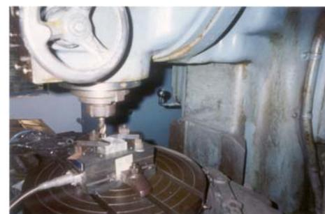
Figure-1(b). Piezo-electric three-component dynamometer (Kistler, type 9257B).
