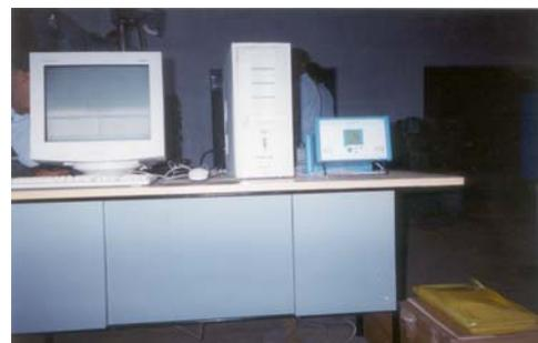
Figure-1(a). Multi channels charge amplifier (Kistler, Type 9403) and a data acquisition system.
