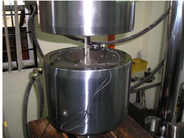
Figure-6. Extensometer installation.
