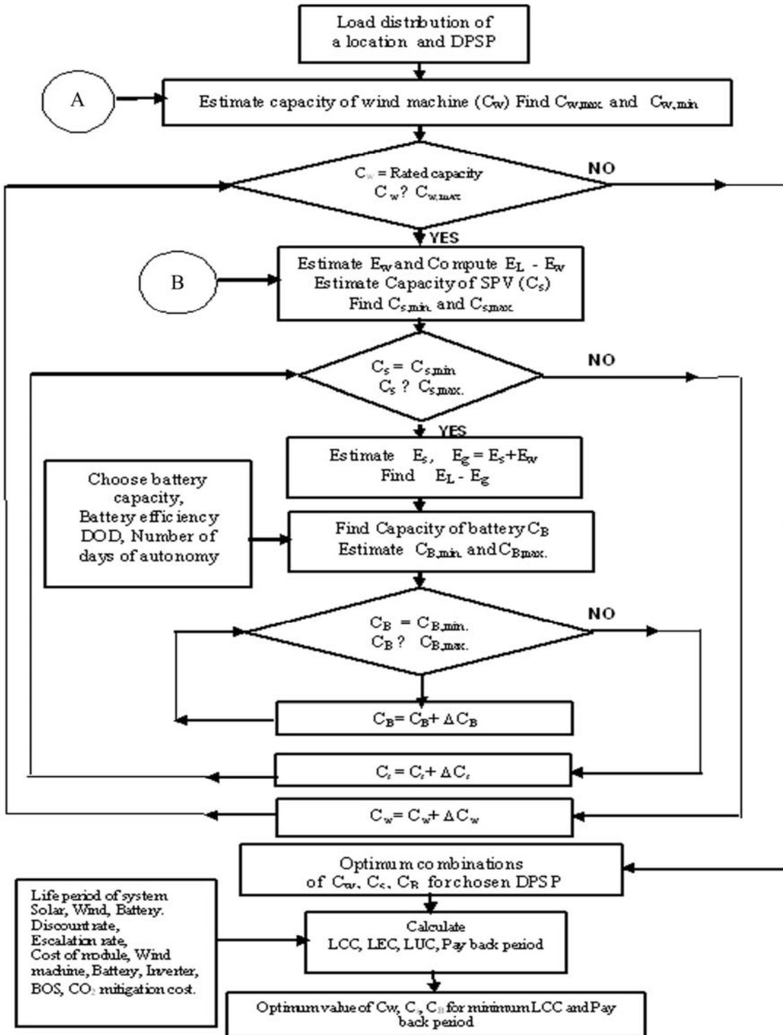
Figure 1 Flow chart for optimization methodology to PV-wind hybrid system
