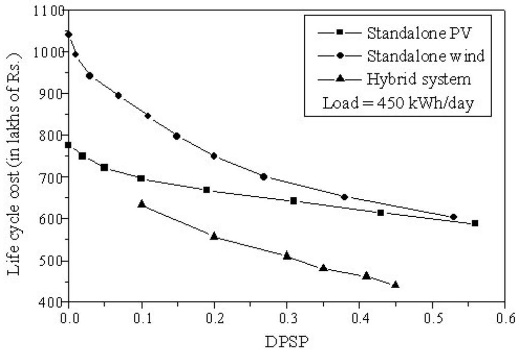
**Figure-4.** Variation of deficiency of power supply probability with respect to life cycle cost for Standalone photovoltaic, wind and hybrid systems at Poompohar.
