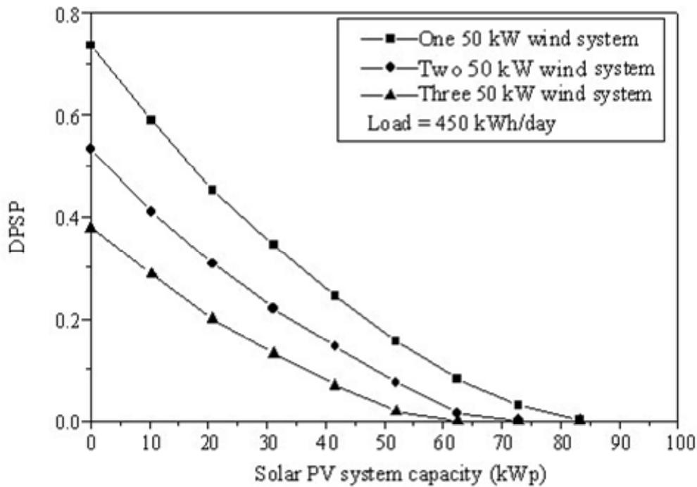
Figure-2. Variation of deficiency of power supply probability with respect to solar PV system capacity at Poompuhar.
