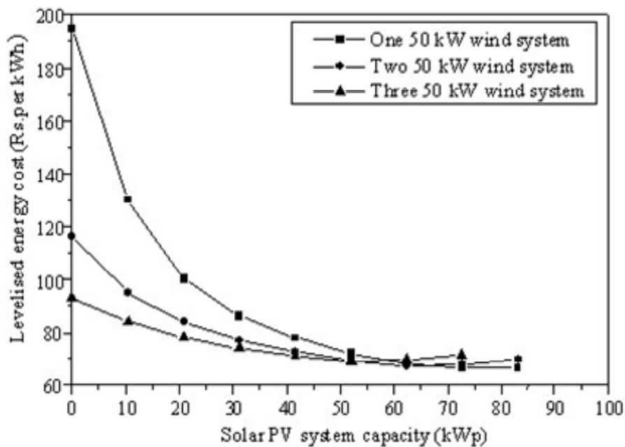
Figure-3. Variation of levelised energy cost with respect to solar PV system capacity with variable wind system capacity for 3 days of battery autonomy at Poompuhar.
