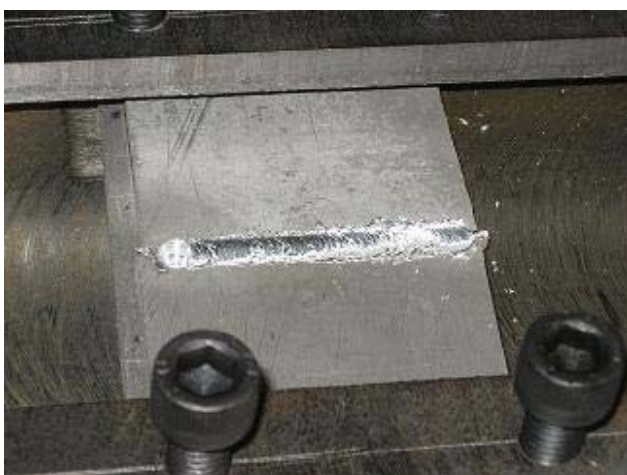
Figure-2. FSW using Makino 3-axis computer numerical controlled milling machine.
