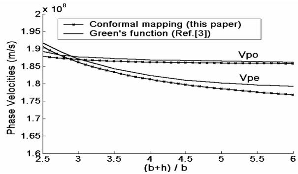
Figure-4. Phase velocities for boron nitride coupler versus  $(b+h)/b$ , ( $w/b = 1.6$ ,  $2s/b = 0.095$ ,  $\epsilon_1 = 5.12$ ,  $\epsilon_2 = 3.4$  at  $\beta = 0$ )
