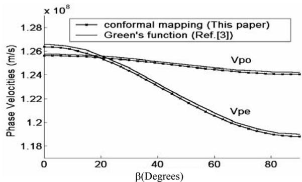
Figure-6. Phase velocities of sapphire substrate versus angle of tilt  $\beta$ , ( $\epsilon_1 = 11.6$ ,  $\epsilon_2 = 9.4$ ,  $h/b = 1.2$ ,  $2s/b = 0.225$ ,  $w/b = 0.69$ ).
