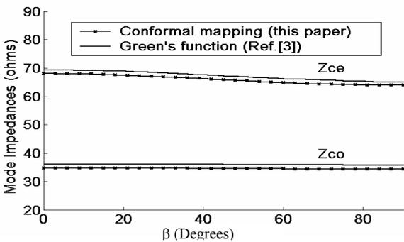
Figure-5. Mode impedances of sapphire substrate versus angle of tilt  $\beta$ , ( $\epsilon_1 = 11.6$ ,  $\epsilon_2 = 9.4$ ,  $h/b = 1.2$ ,  $2s/b = 0.225$ ,  $w/b = 0.69$ ).
