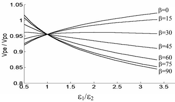
Figure-3. Phase velocity ratio versus anisotropy ratio with angle of tilt  $\beta$  as a parameter ( $\epsilon_2 = 3.78$ ,  $2s/b = 0.25$ ,  $h/b = 10$ ,  $w/b = 0.1$ ).
