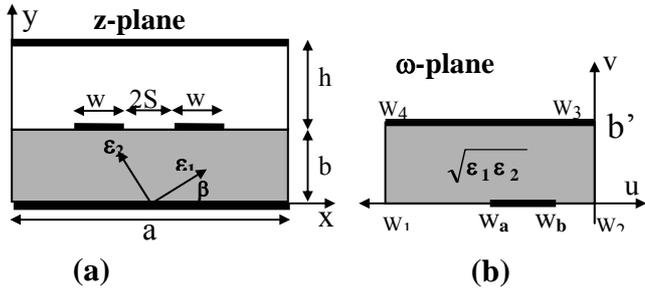
Figure-1. (a) Shielded coupled microstrip lines; (b) lower left part (flipped vertically).
