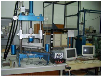
Figure -2b. Complete assembly of the flexural test.
