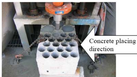
Figure-2. Extraction of core specimen.
