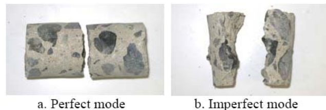
Figure-3. Failure mode of PLT specimen.
