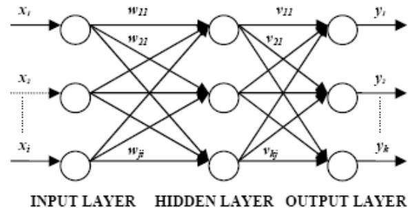
Figure-1. Three layered neural network.
