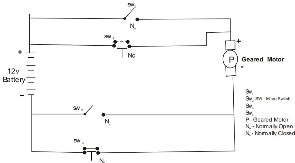
Figure-2. Tipping bucket operational circuit system diagram.
