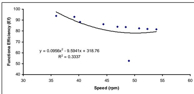
**Figure-8.** Functional efficiency curve at angle  $7^{\circ}$ .
