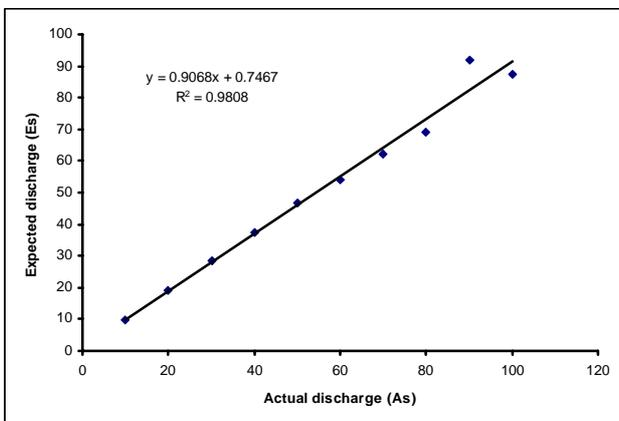
**Figure-4.** Linear relationship of expected discharge ( $E_s$ ) against actual discharge ( $A_s$ ) in  $m^3/s$  at angle  $5^0$ .
