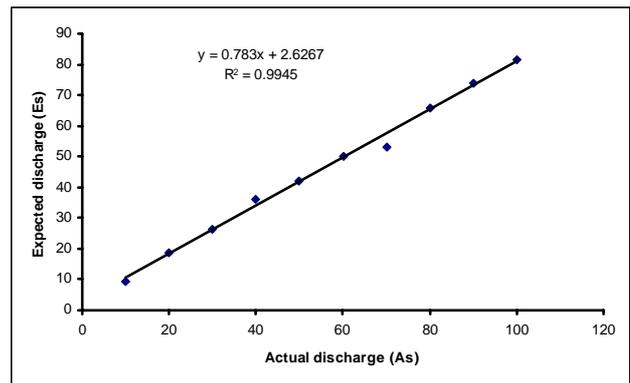
**Figure-5.** Linear relationship of expected discharge ( $E_s$ ) against actual discharge ( $A_s$ ) in  $m^3/s$  at angle  $7^0$ .
