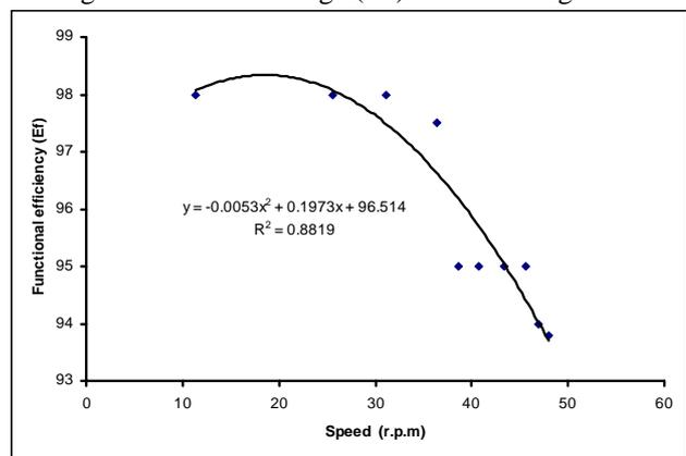
**Figure-6.** Functional efficiency curve at angle  $3^0$ .
