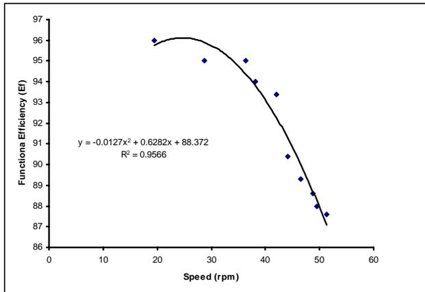
**Figure-7.** Functional efficiency curve at angle  $5^{\circ}$ .
