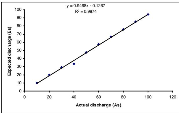
**Figure-3.** Linear relationship of expected discharge ( $E_s$ ) against actual discharge ( $A_s$ ) in  $m^3/s$  at angle  $3^0$ .
