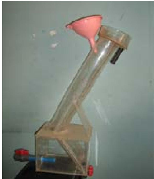
Figure-6. The simple classifier used for fine iron minerals recovery from itakpe plant tails.
