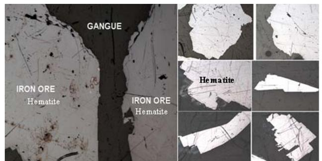
Figure-4. Micrographic appearance of the itakpe iron ore at x 40 magnifications.
