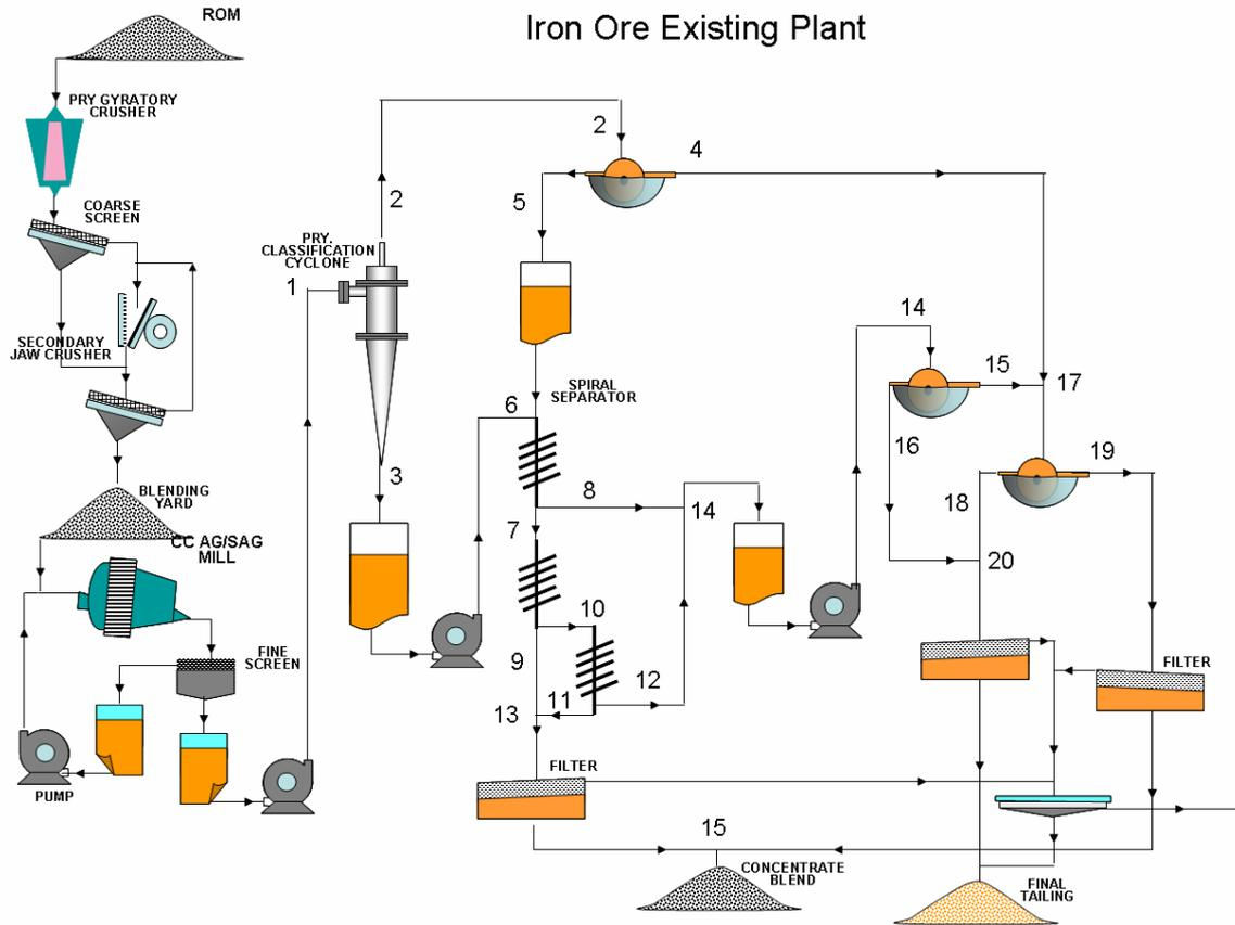
Figure-5. Simplified process flowsheet of Itakpe iron ore processing plant.
