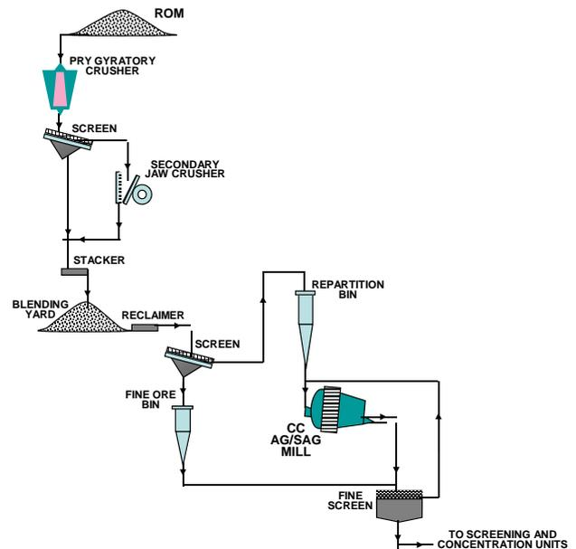
**Figure-8.** Preferred comminution circuit for preparation of suitable feed.
