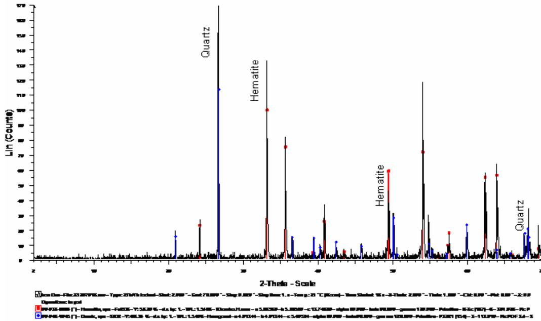
Figure-1. An XRD diffraction curve the iron ore showing major mineral types.
