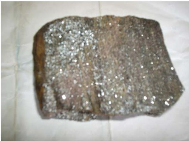
Figure-2. As-mined appearance of as-mined grain dissemination iron ore showing coarse grain dissemination.
