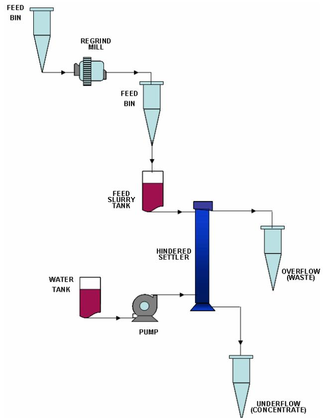
Figure-7. Flow Circuit for recovery of the hindered settling process.
