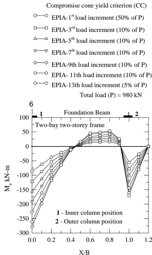
Fig. 3 Variation of BM's in foundation beam for elasto-plastic analysis
