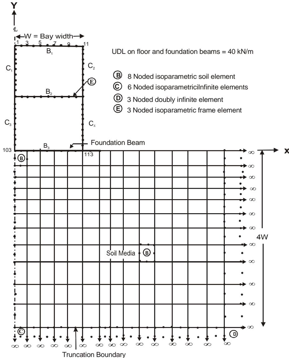
Boundary Conditions: All nodes on the line of symmetry are restrained in x-direction
