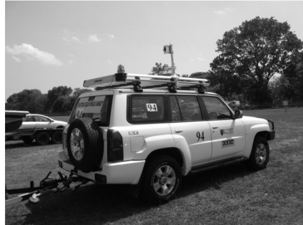
Figure-9. Data acquisition and telemetry system of solar vehicle road test.
