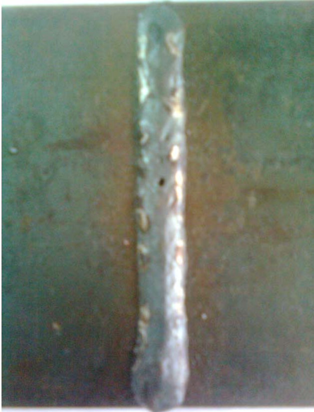
Figure-3. Typical TIG welded coupon with overlap and porosity.
