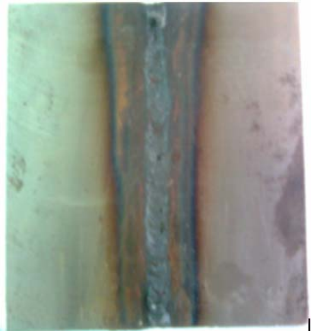
Figure-6. Typical MIG welding with under fill and porosity.
