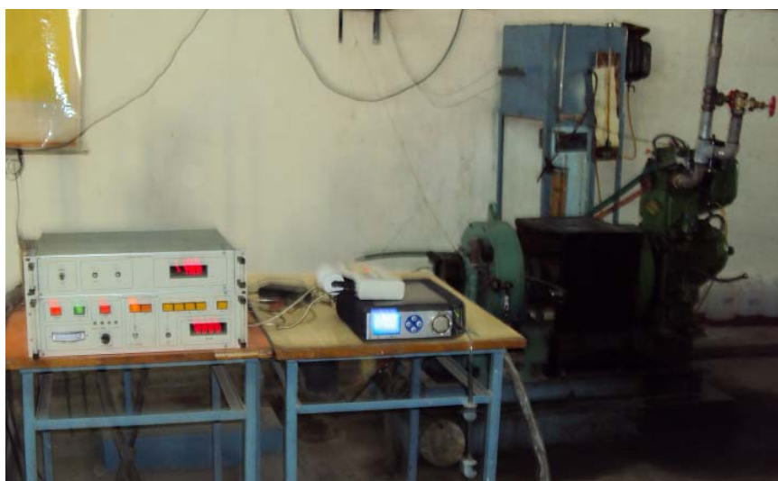
Figure-1. Experimental setup showing eddy current dynamometer, controller and gas analyzer.
