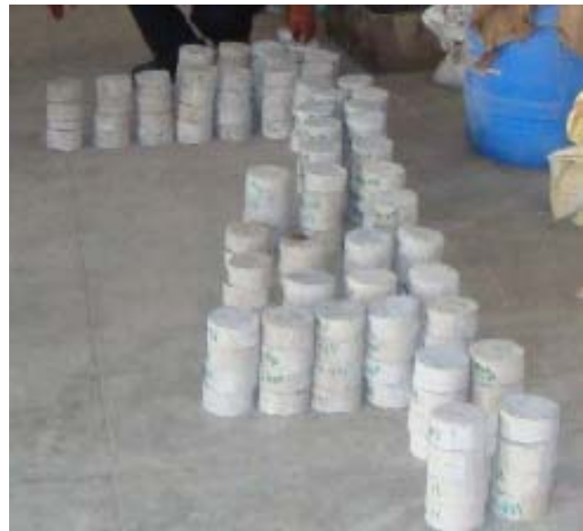
Figure-2. Typical M20 grade specimen with varying % of GFRC.
