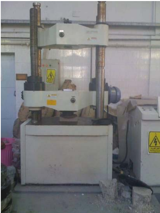
Figure-6. The Shumadsu machine used for testing the cementitious straw bricks.
