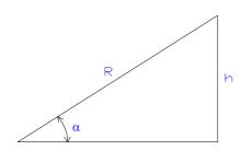
New clearance or required clearance,  $\theta^1 = \theta + \alpha = \theta + \sin^{-1}(h/R)$  and
