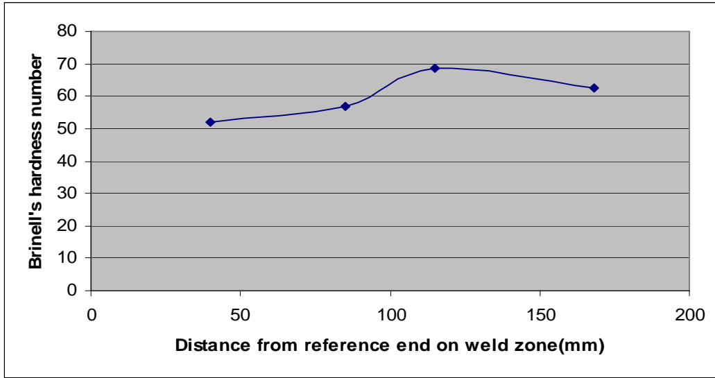
Figure-14. Variation of Brinell's hardness number with distance along the weld zone.
