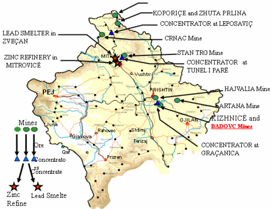
Figure-1. Map of Kosovo showing TREPÇA mines concentrators and final processing facilities.
