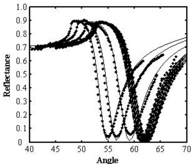
**Figure-2.** SPR signal for biodiesel mixture prepared from volume percentage of palm oil was from 2.5% to 90%. (● is experimental data and solid line is fitted.)
