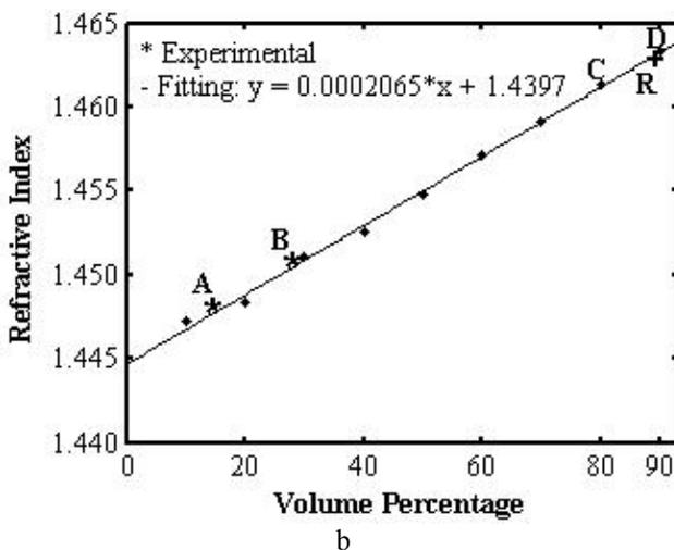
**Figure-3.** Refractive index of the respective volume percentage of palm oil in the biodiesel mixture. ( $\cdot$  is experimental data and solid line is fitted.)
