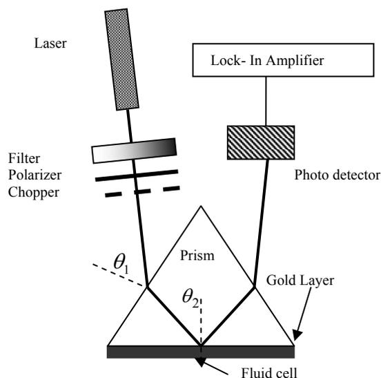
**Figure-1.** Experimental set up (He-Ne laser, filter, polarizer, prism, photo detector, fluid cell, lock in Amplifier).
