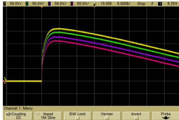
Figure-10. Per unit surge voltages with MOV provided across 50% of the winding length at nodes 1, 2, 3 and 4 to ground with respect to time ( \alpha = 11.8 ).
