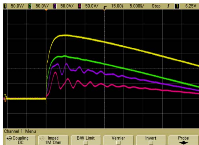
Figure-11. Per unit surge voltages with MOV provided across 50% of the winding length at nodes 1, 5, 6 and 7 to ground with respect to time ( \alpha = 11.8 ).
