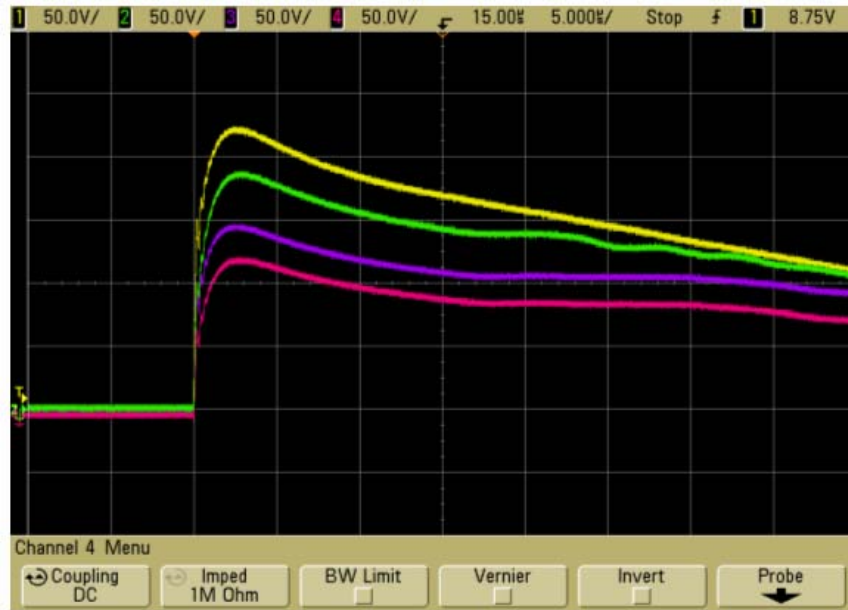
Figure-19. Per unit surge voltages with Non-Identical MOV provided across 100% of the winding length at different nodes 1, 2, 3 and 4 to ground with respect to time ( \alpha = 18.9 ).
