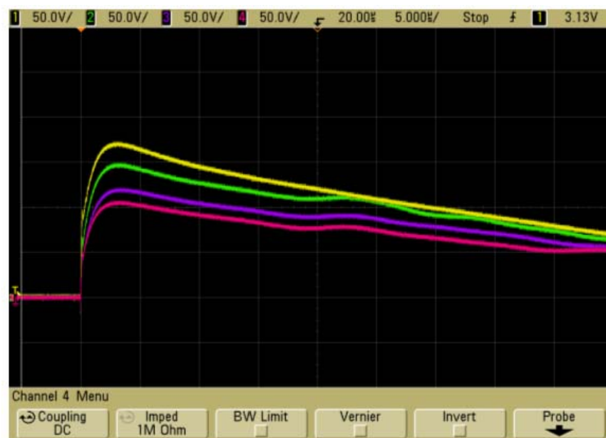
Figure-13. Per unit surge voltages with MOV provided across 100% of winding length at nodes 1, 2, 3 and 4 to ground with respect to time ( \alpha = 11.8 ).
