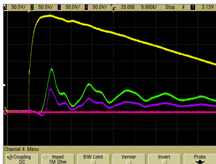
Figure-9. Per unit surge voltages at different nodes to ground 1, 7, 8 and 9 with respect to time without MOV ( \alpha = 11.8 ).
