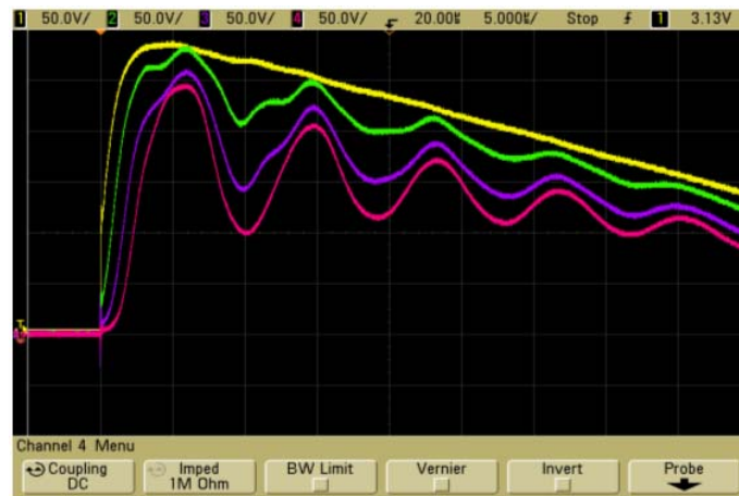
Figure-7. Per unit surge voltages at different nodes to ground 1, 2, 3 and 4 with respect to time without MOV ( \alpha = 11.8 )
