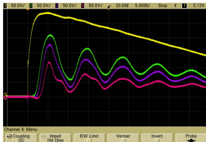
Figure-8. Per unit surge voltages at different nodes to ground 1, 5, 6 and 7 with respect to time without MOV ( \alpha = 11.8 ).
