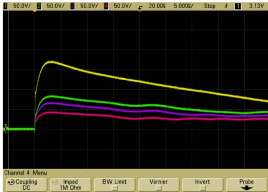
Figure-14. Per unit surge voltages with MOV provided across 100% of winding length at nodes 1, 5, 6 and 7 to ground with respect to time ( \alpha = 11.8 ).
