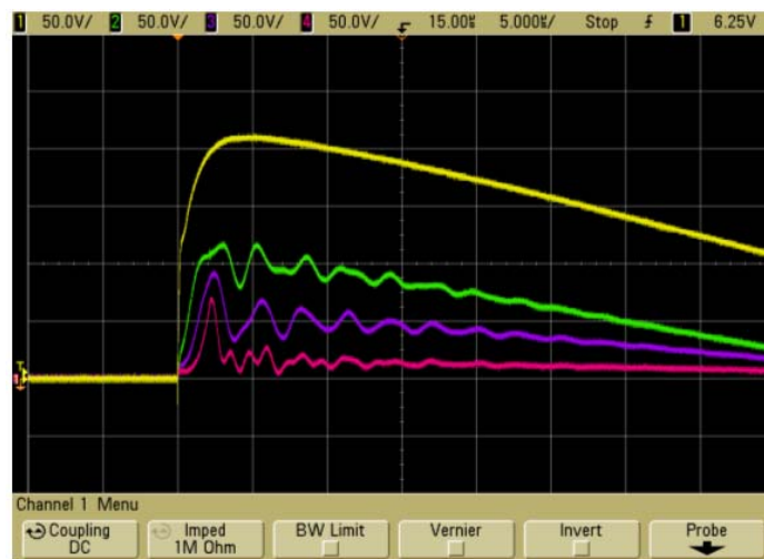
Figure-12. Per unit surge voltages with MOV provided across 50% of the winding length at nodes 1, 6, 7 and 8 to ground with respect to time ( \alpha = 11.8 ).
