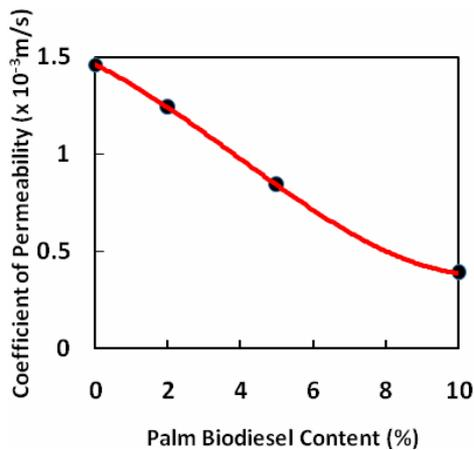
**Figure-7.** Variation of coefficient of permeability with palm biodiesel content.
