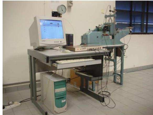
**Figure-2.** Modified computer-controlled simple shear apparatus.
