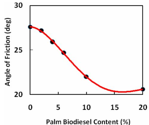
**Figure-5.** Variation of friction angle with palm biodiesel content ( $D_r=30\%$ ).
