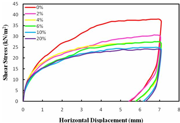
**Figure-3.** Stress-displacement relationship for 30 KPa normal stress ( $D_r=30\%$ ).
