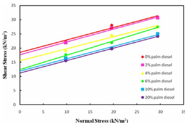
**Figure-4.** Failure envelopes for clean and contaminated soils ( $D_r=30\%$ ).
