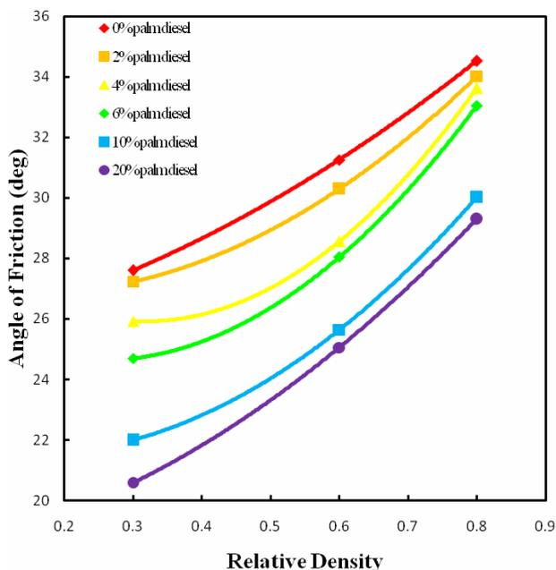
**Figure-8.** Variation of friction angle with relative density.
