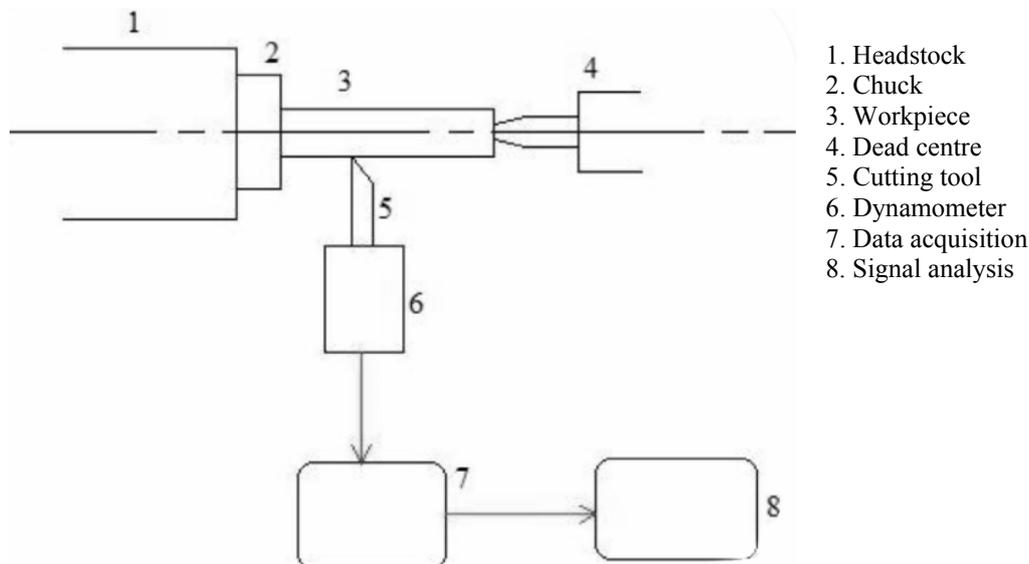
**Figure-9.** Scheme of experimental setup.
