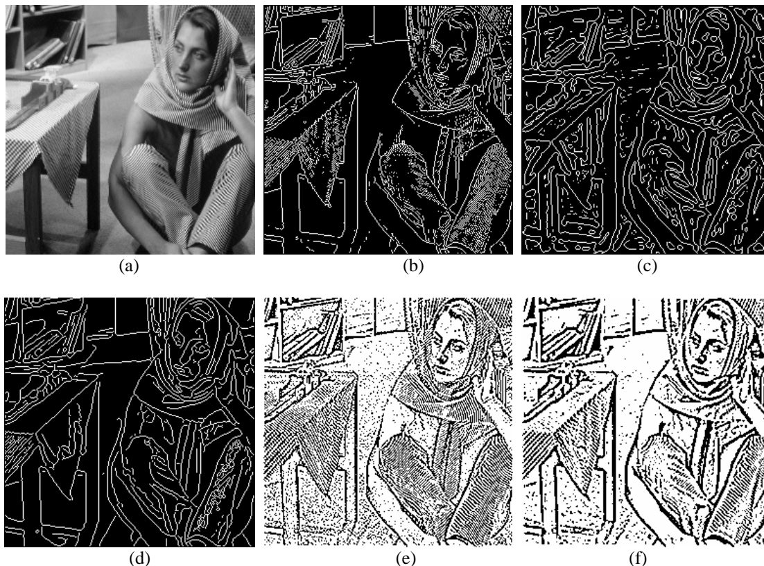
Figure-1. Performance of edge detectors on Barbara image. (a) Original Image, (b) Sobel, Thr=11, (c) LOG, Thr=0.25, (d) Canny, Thr= [0.0115, 0.1175] (e) Mask B, Thr=122 and (f) Mask B2, Thr=115.
