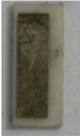
Figure-1. Double chip mask pattern (2 mm x 6 mm).
