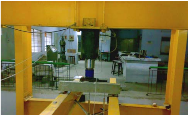
Figure-2. Beam and LVDT arrangement in 100 ton loading frame.
