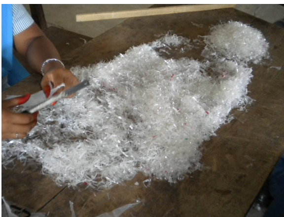
Figure-1. Waste domestic plastics are made into fibre.
