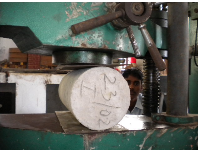
Figure-5. Split tensile strength testing on cylinders.
