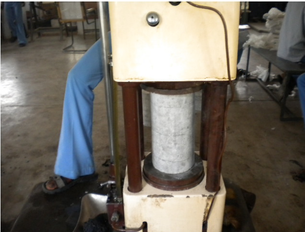
Figure-4. Compressive strength testing on cylinders.
