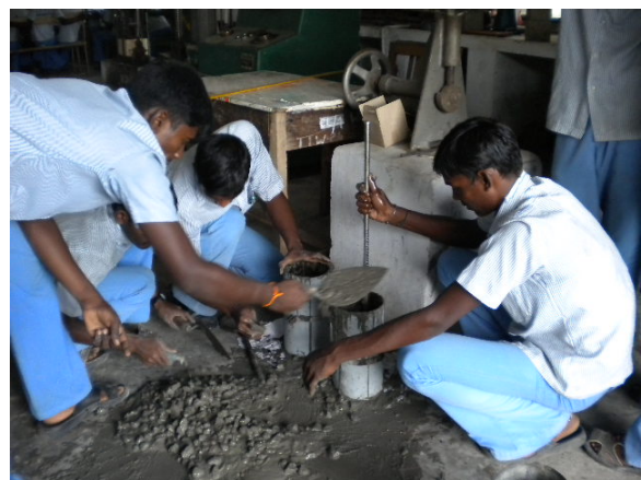
Figure-2. Casting of cylinders.
