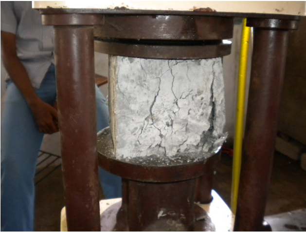
Figure-3. Compressive strength testing on cubes.
