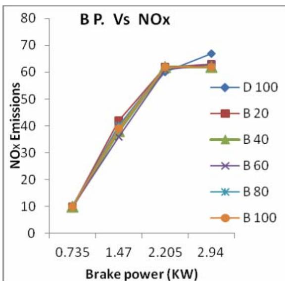
Figure -6. NO<sub>x</sub> Vs brake power.
