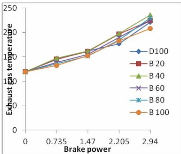
Figure -5. Exhaust gas temp. Vs brake power.
