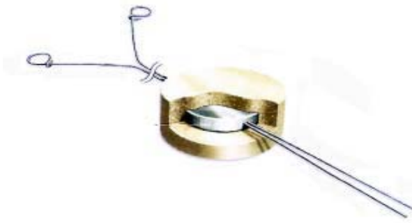
Figure-6. Typical cut-away view of galvanic anode.
