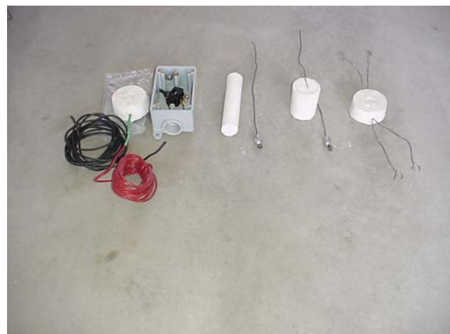
Figure-5. Typical view of the galvanic anodes and monitoring box.
