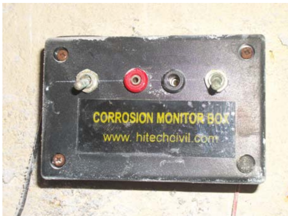
Figure-12. A view of corrosion monitoring box.
