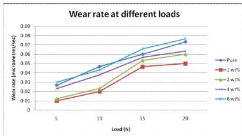
Figure-7. Variation of wear rate with Load for different % of Nano ZnO.
