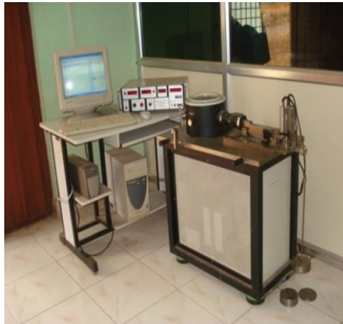
Figure-1(a). Pin on disc set-up.
