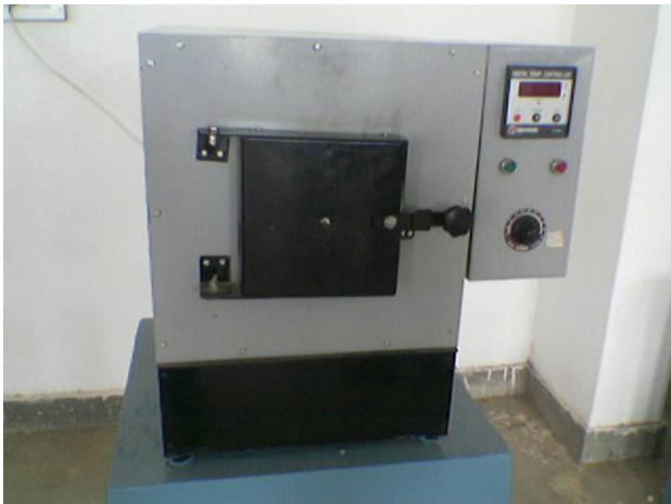
Figure-7. Sintering furnace.
