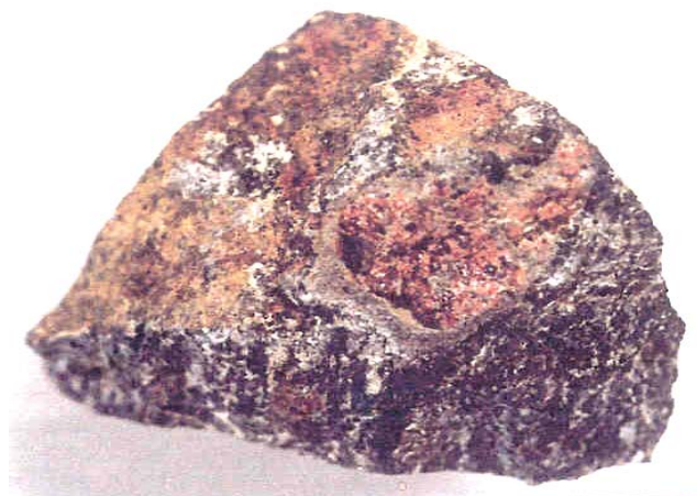
Figure-2a. Garnet-diopside amphibolite schist (garnet porphyroblasts size of 2.5 cm with kelyphitic rim one around the garnets).
