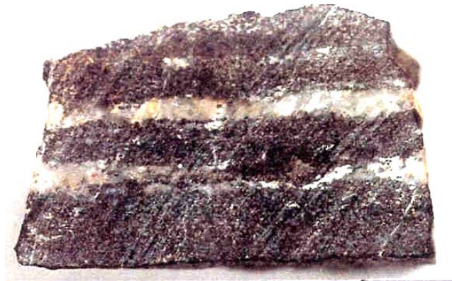
Figure-2b. Garnet-diopside amphibolite slate with banded of fresh plagioclase.
