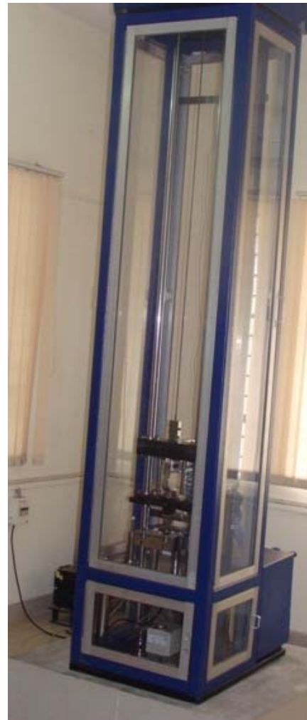
Figure-2. Falling weight impact test equipment.
