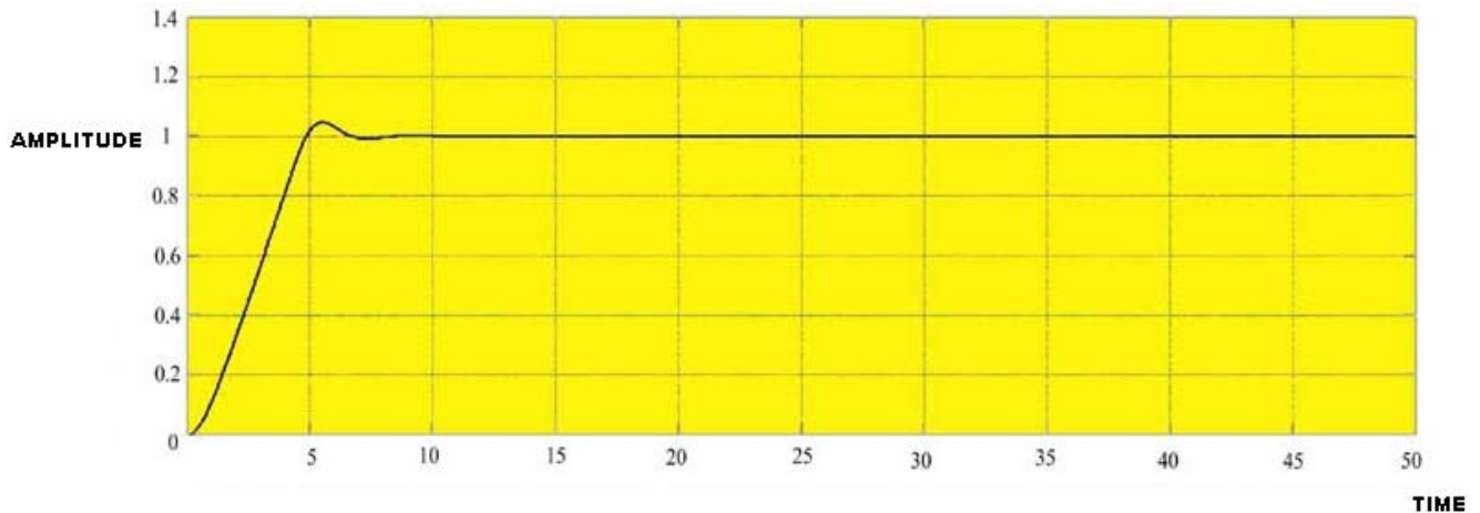
Output as seen on Scope with FPGA based digital PID
