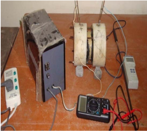
Figure-3. Test setup for permeability test of concrete.
