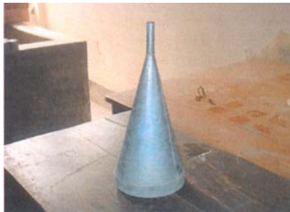
Figure-2. Flow cone and its dimensions.
