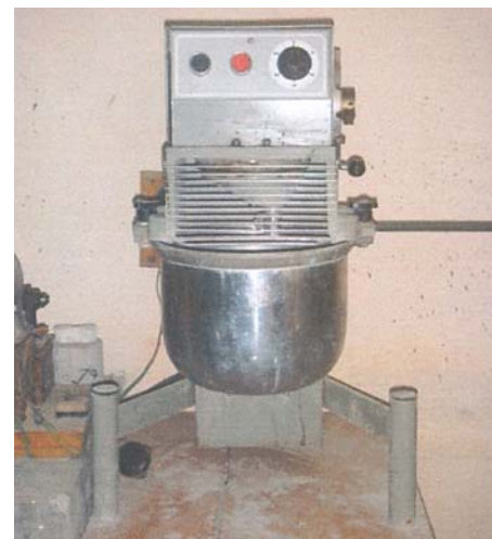
Figure-1. Grout mixture machine.
