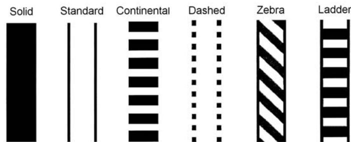
Figure-8. Typical sidewalk crossing signs.
