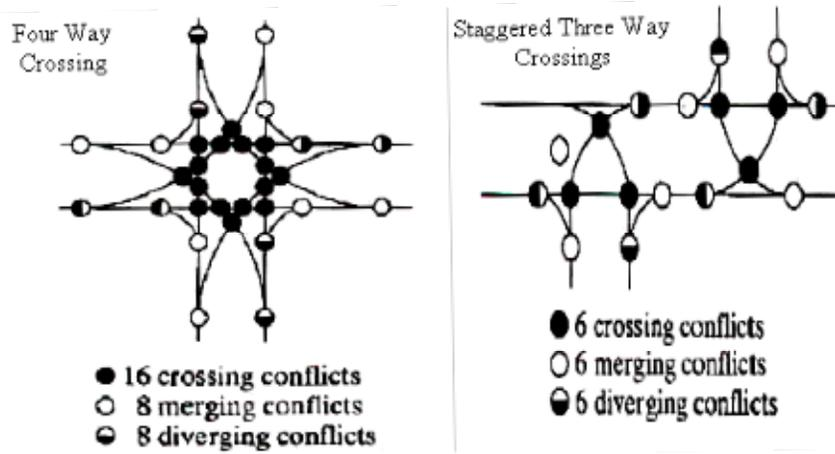
Figure-10. Four way crossing versus staggered three way crossings.
