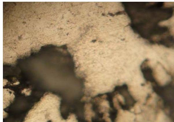
Figure-3. Optical microscopy of aluminum silicon carbide composite shows particle clustering.
