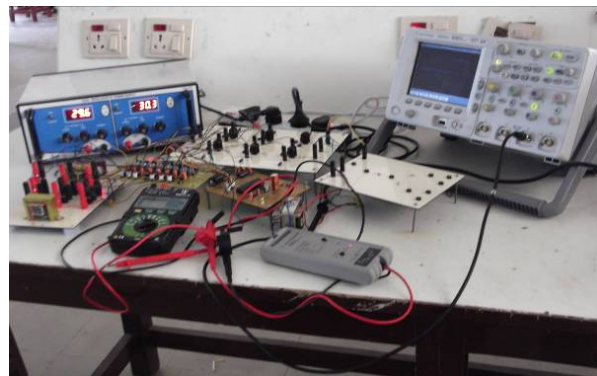
Figure-17. Hardware setup including both power circuit and control circuit.
