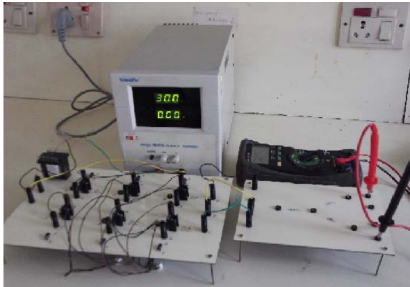
Figure-15. Hardware setup of three-phase CSI.
