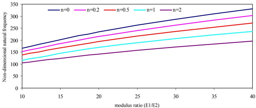
**Figure-4.** Non-dimensionalized natural frequencies Vs modulus ratio (E1/E2) for a simply supported FGM plate for model.
