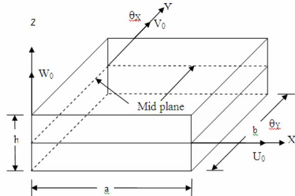
**Figure-1.** Geometry of FGM plate along with reference axis and displacement components.
