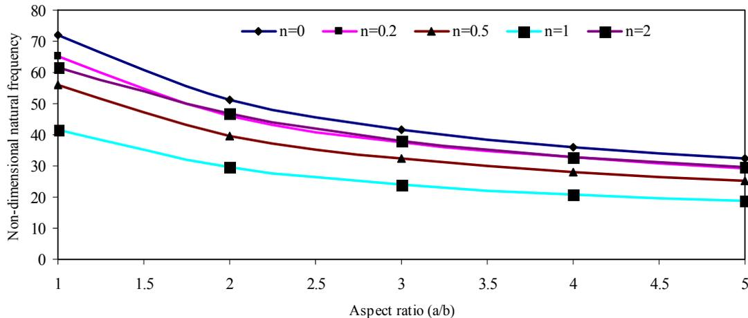
**Figure-5.** Non-dimensionalized natural frequencies Vs aspect ratio (a/b) for a simply supported FGM plate for model.
