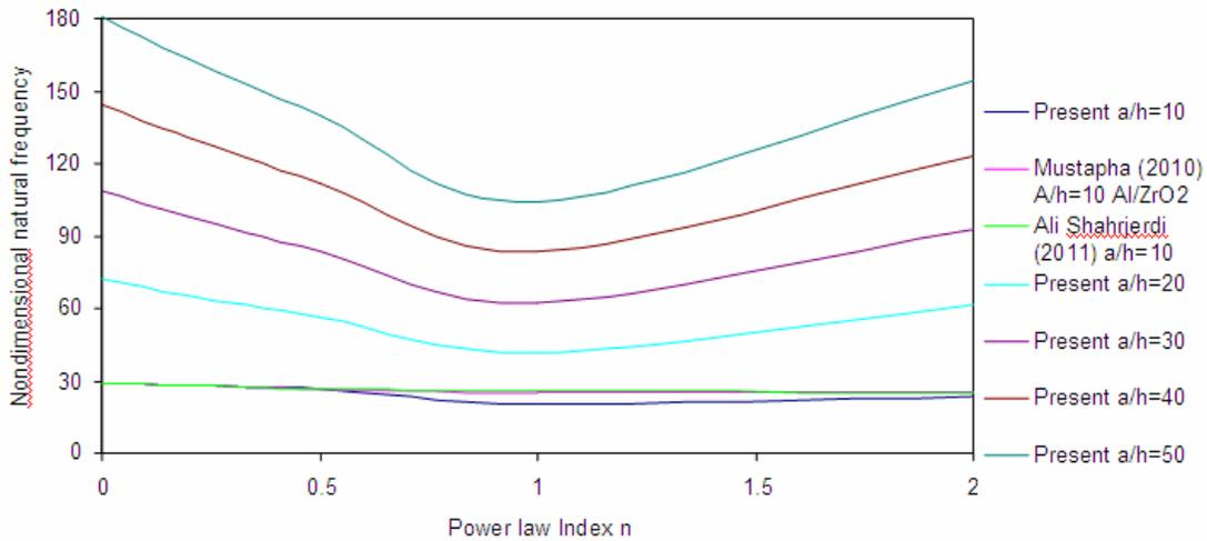
**Figure-2.** Non-dimensionalized natural frequencies Vs Power law index n with different side to thickness ratio's for a simply supported FGM plate.
