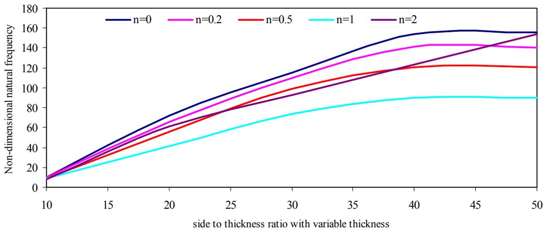
**Figure-3.** Non-dimensionalized natural frequencies Vs side to thickness ratio (a/h) for a simply supported FGM plate with variable thickness for model.
